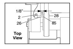
Screw (2) and move the Reed Switch slightly. Retighten the Screw. Re-attach the hood, and run the treadmill for a few minutes to check for a correct speed reading.
